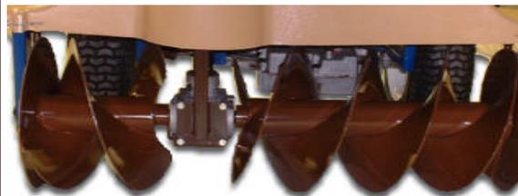
The 4+ inch opening in the auger means that the heads can pass through without damage even if they are above ground
